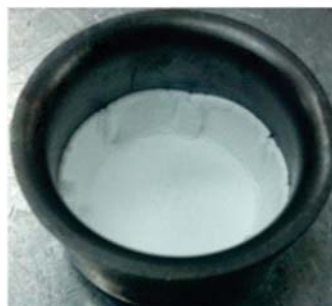
Figure 1. Use a rod or other wide, round-ended object to evenly place the filter into the crucible.
